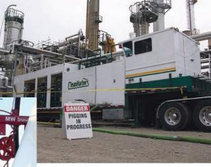
Clean Harbors' closed loop pigging process uses a high-volume, low-pressure water pumping system to propel its patented bi-directional pigs through pipes and coils to effect cleaning.
